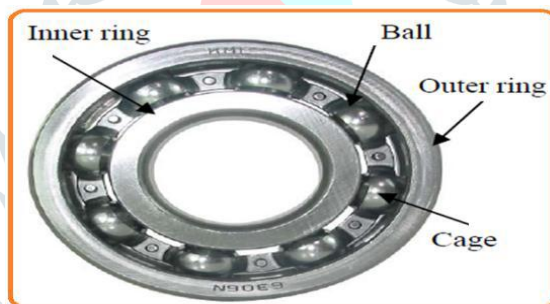
Figure 1. Deep Groove Ball Bearing.
