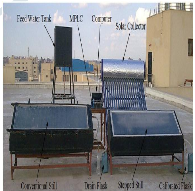
Fig. 7.1 Experimental setup of solar still.
