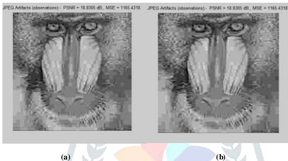
Fig-1 : Compressed image with visible artifacts at a) Q=8 and b) Q=10
