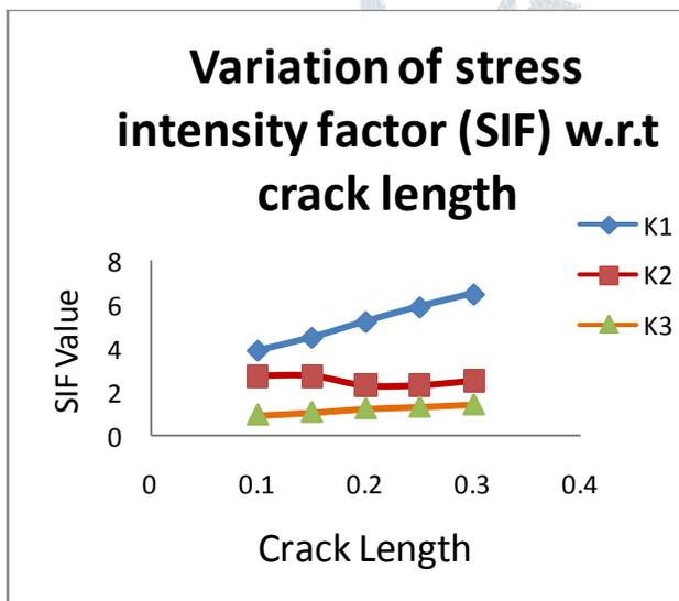
Figure– Variation of stress intensity Factors w.r.t crack length
