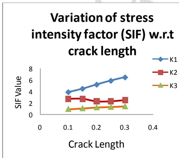
Figure– Variation of stress intensity Factors w.r.t crack length
