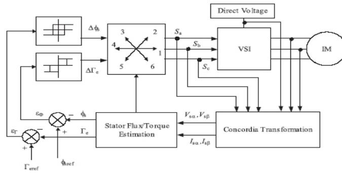
Fig.1 Block diagram of DTC scheme
