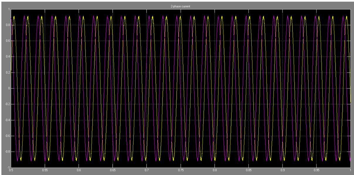
Fig 4.13 : 2-phase current in DTC with FLC model
