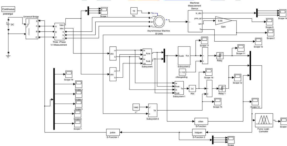
Figure 4.8 : Direct Torque Control of Induction Motor with Fuzzy Logic Controller Schematic using SIMULINK/MATLAB.
