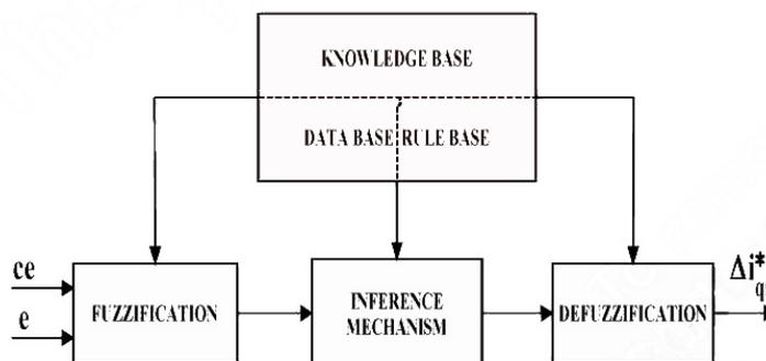
Fig: Block diagram for The fuzzy logic
