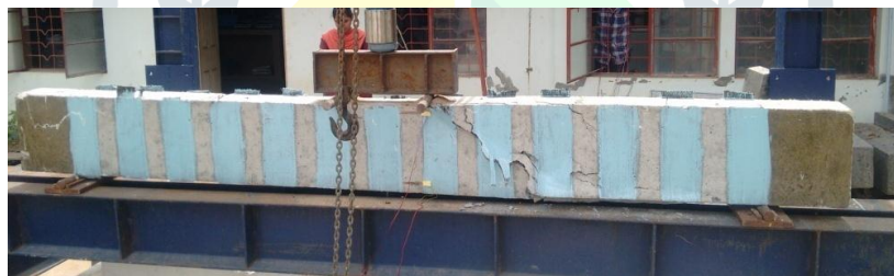
Fig. 9.Failure mode of U -wrap strip beam -1
