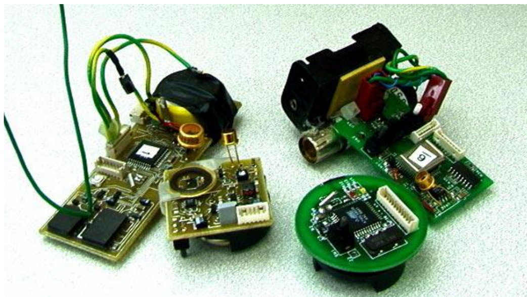
Figure 2: COTS Motes. From left to right: RF Mote, CCR Mote, we C Mote, Laser Mote.
