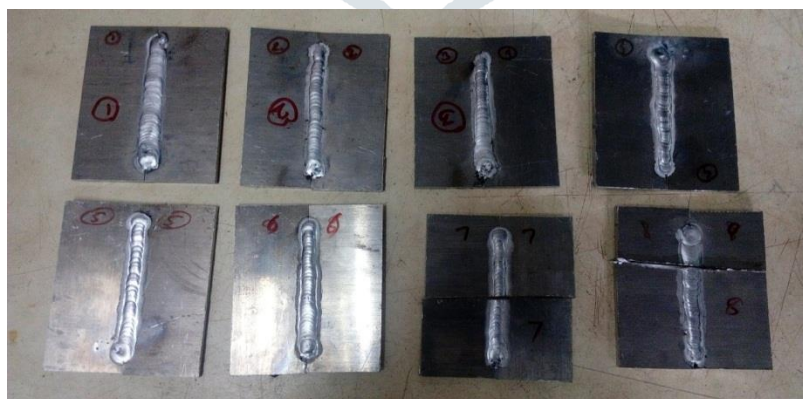
Image of AA 6082 welded samples using GTA Welding
