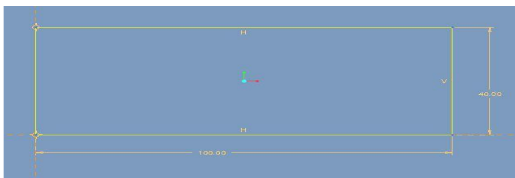
Fig 1.2 Design of AA 6082 plate specimen
