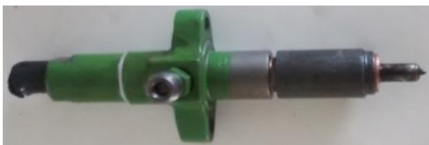
Figure3: Diesel Engine Fuel Injector
