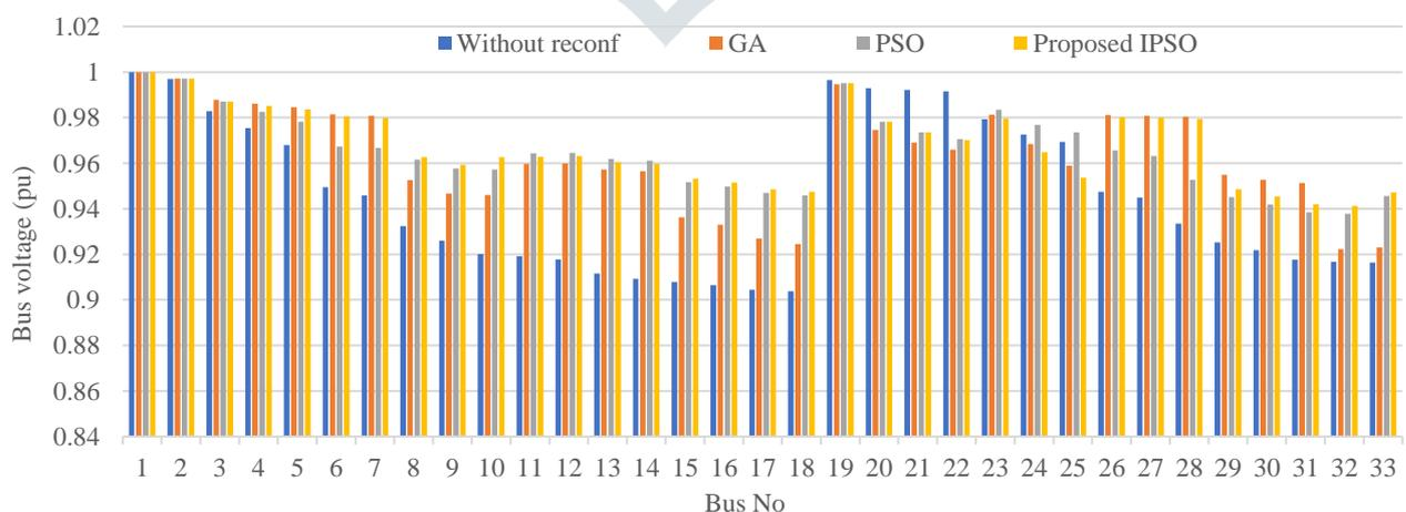
Fig.1 Comparison of bus voltage after reconfiguration using GA, PSO and the proposed IPSO algorithms
