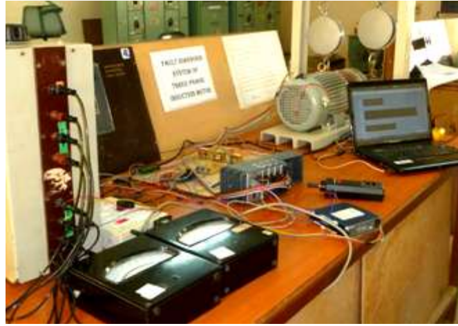
Figure 2 Experimental setup of cRIO based Induction Motor Diagnosis
