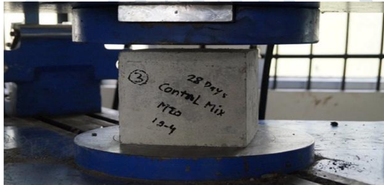
Figure.4 Compressive Strength test of cube samples in UTM
