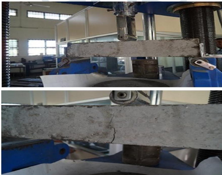
Figure.5 Flexural Strength tests of beam samples in UTM
