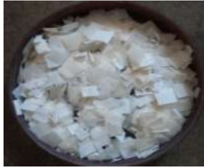
Figure 1 Square Pieces of Plastic Waste of Milk Polythene Admixture
