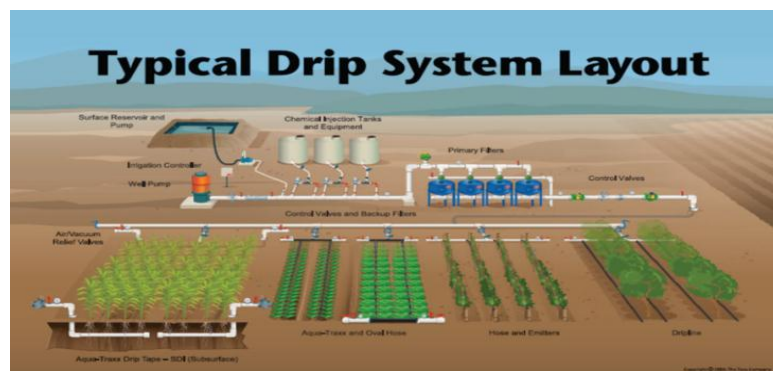
Figure 1: Typical Drip Irrigation
