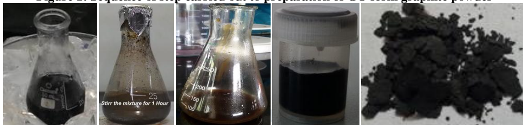
Figure 1: Sequence of step carried out to preparation of GO form graphite powder
