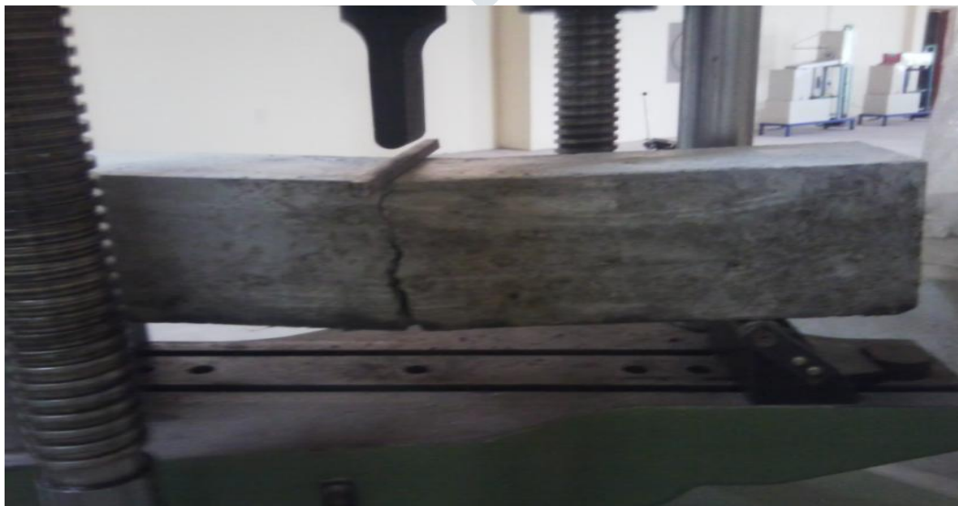
Figure3: Flexural Strength Test
