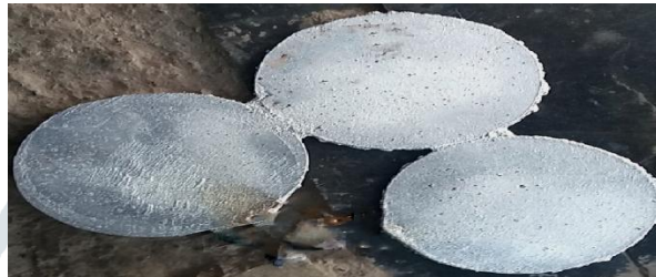
Figure-7.2: Composite specimen for 2%,6%,10% of volume fraction of thermal conductivity test
