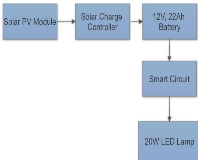
Figure 1: Working Block Diagram
