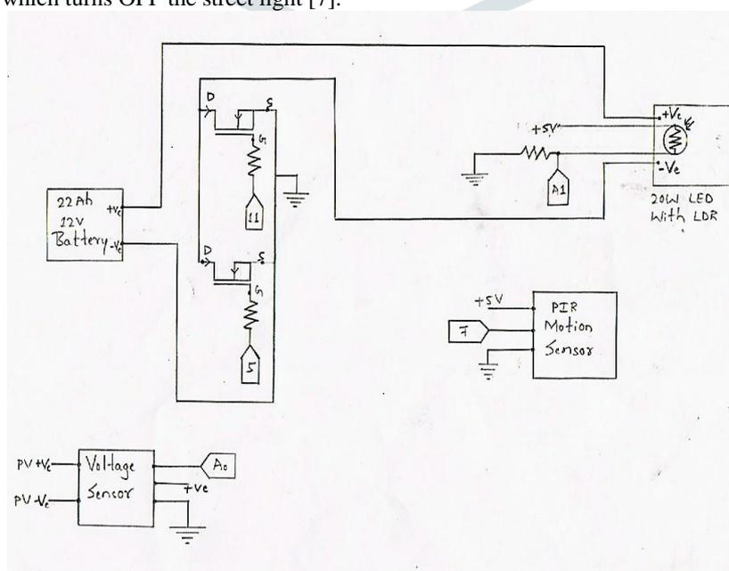
Figure 2: Circuit diagram for smart circuit
