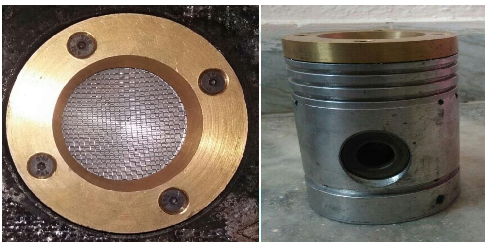
Fig.2. Piston with meshed bluff bodies and brass crown piston
