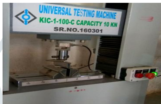
Figure no: 4 ILSS test set up
