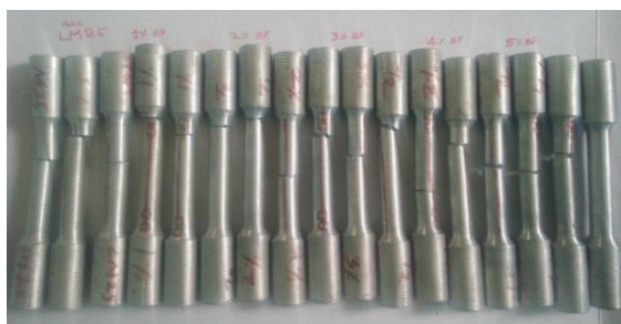
Figure 3.4 Tensile test specimens after testing.
