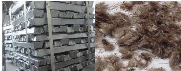
Figure 2.1 Al alloy LM25 Ingots and Short basalt fibers.
