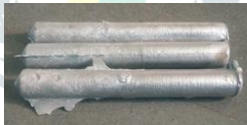
Figure 3.2 casted cylindrical composite ingot
