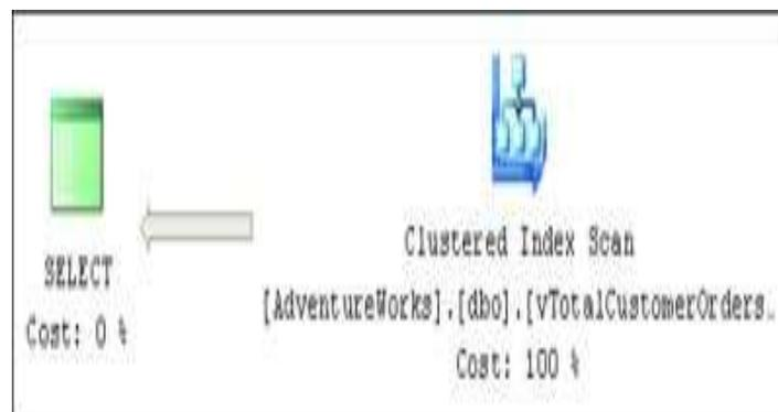
Fig. 6 Execution plan when using indexed view
