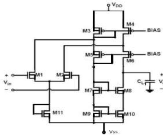
**Figure 1:** Transistor level circuit diagram of Folded Cascode Operational Amplifier
