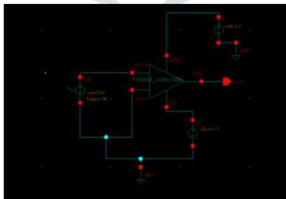
**Figure 2:** Test setup of folded cascode op-amp in cadence
