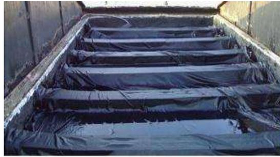
**Fig.8** Kalidasa’s still with aluminium fin covered with black cloth in the basin
