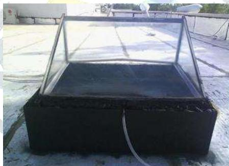
**Fig.6** Tabrizi's double slope solar still
