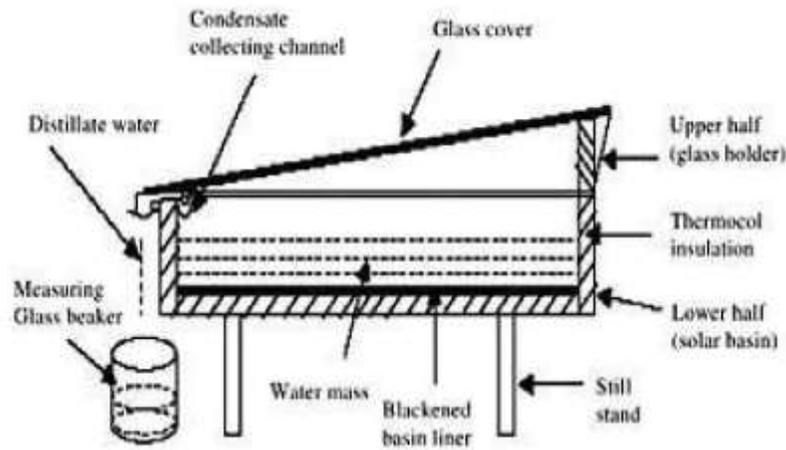
Fig.1 Schematic diagram of Sahoo et al. solar still
