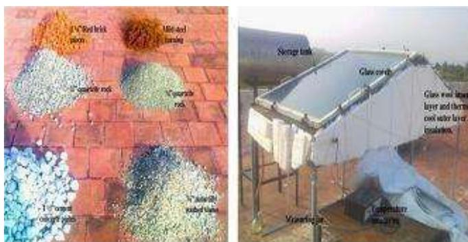
**Fig.7** Different storage material and still used By Kalidasa Murugavel
