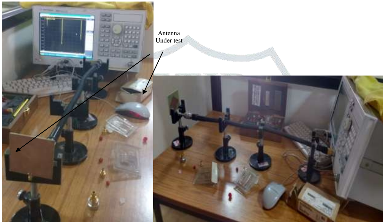
Figure 3. Setup for the measurement of return loss and VSWR.
