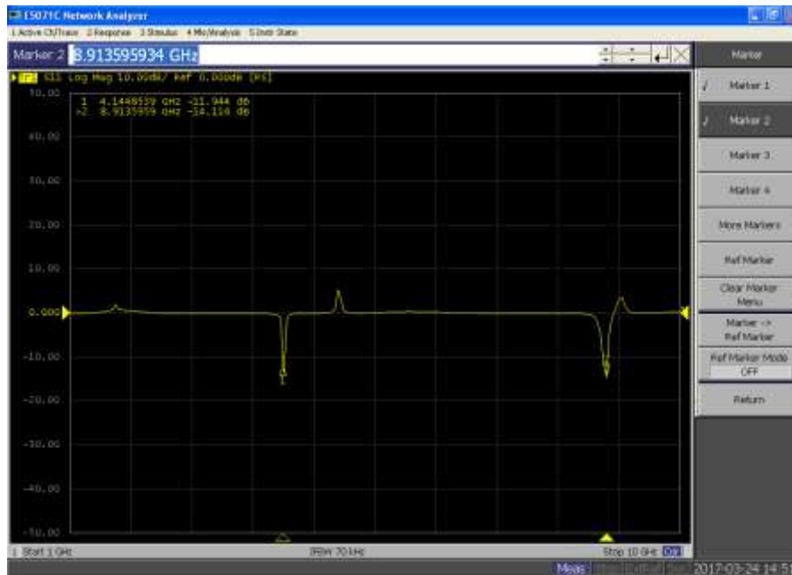
Figure 5. Practical Return loss for square patch with tail feed.
