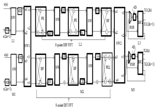
Fig.2: Proposed 16-Point Radix-2 Fft Architecture with Outputs In Natural Order
