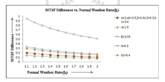
Figure indicates that MTSF difference (MODEL I-MODEL II) decreases with increase of normal weather rate ( $\beta_1$ ) and failure rates ( $\lambda$  and  $\lambda_1$ ) of the units. But, it increases with the increase of abnormal weather rate ( $\beta$ ) and repair rate ( $\alpha$ ) of the main unit. Thus, the study reveals that the idea to allow operation of the system in abnormal weather is not useful in improving reliability of the system.
