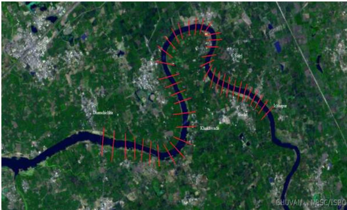
Figure 1: Study Reach with Cross-Sectional Details
