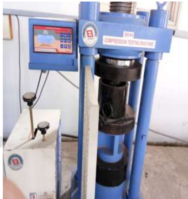
Fig 1 compression testing equipment
