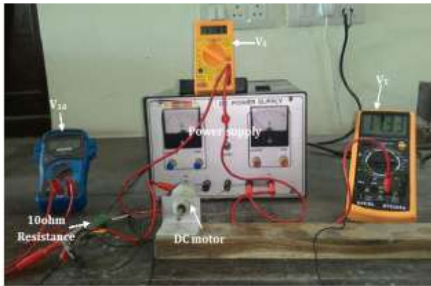
(a) Figure 3: The experimental setup for: (a) no external load characteristic; (b) stall condition.
