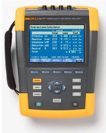
Figure 7. Fluke power quality meter.
