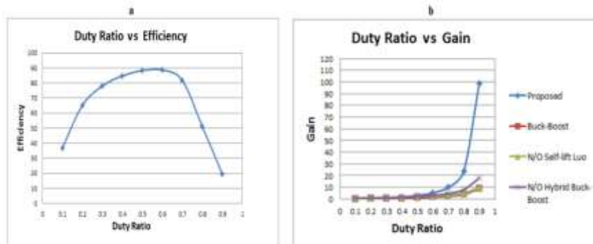
Fig. 15. (a) Efficiency versus duty ratio (b) Gain versus duty ratio
