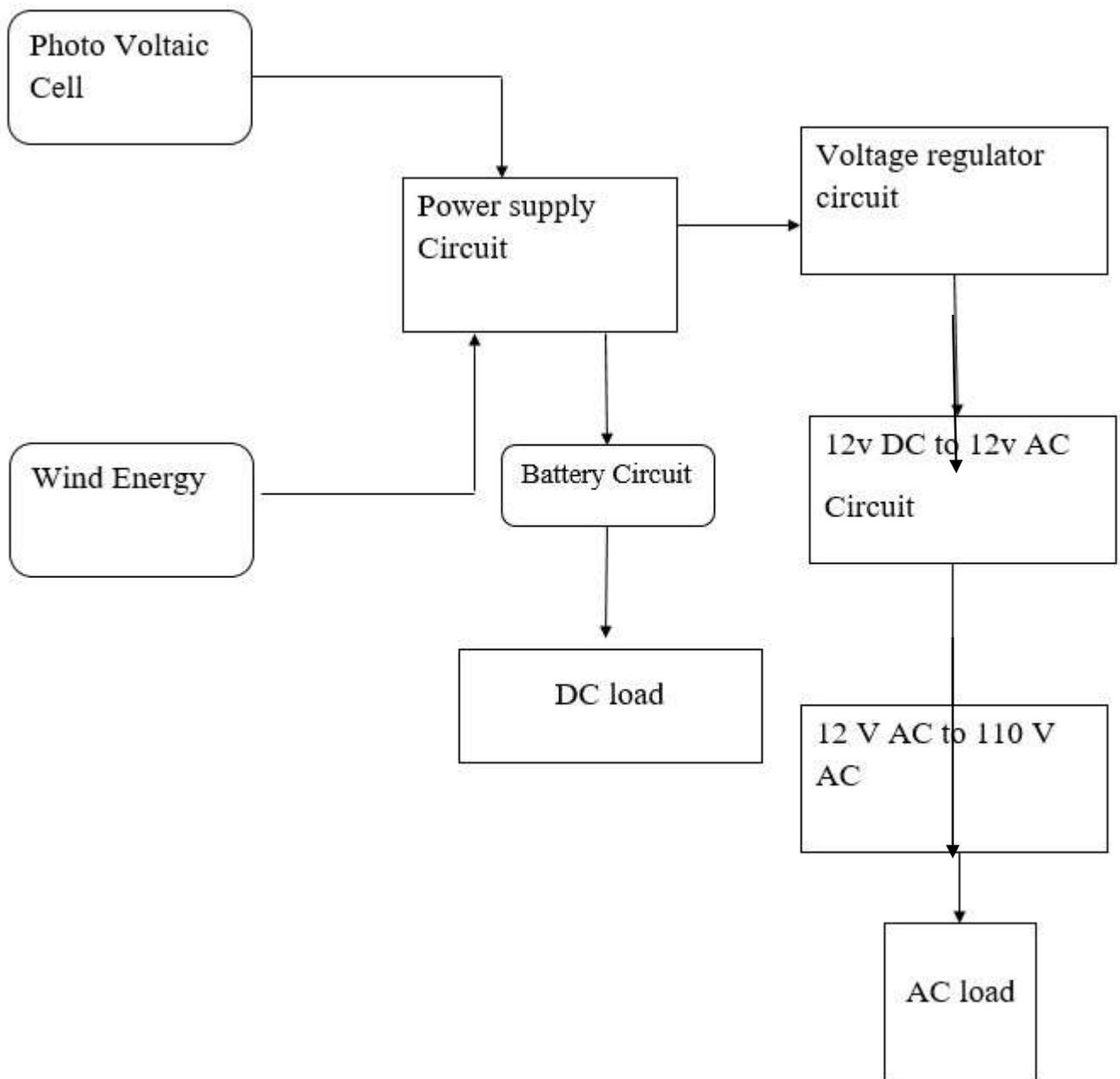
Fig1. Block diagram of proposed system
