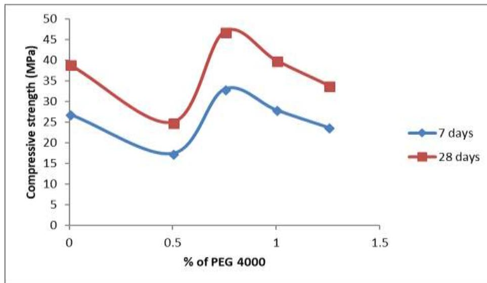
Figure 4. Variation of Compressive Strength with varying %age of PEG-4000 for 7 and 28 days.
