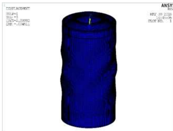
Figure.16: Buckling Mode Shape
