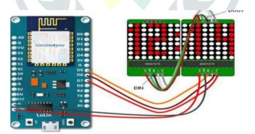
Hardware wiring from Arduino to dot matrix display data pin D5 from arduino is connected to the display pin Din.
