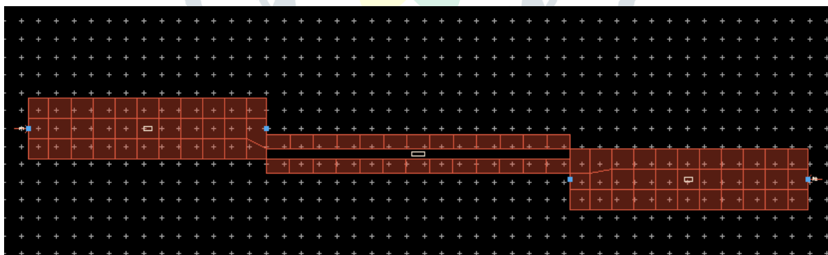
Figure 14: Band pass filter realisation through layout design
