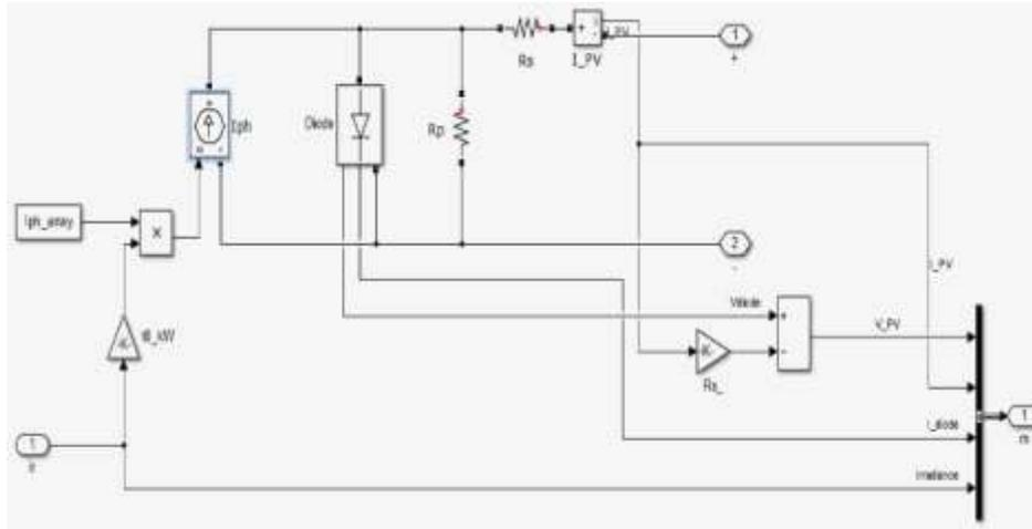
Fig 1: internal circuit of pv array in matlab.
