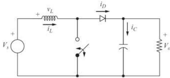
Fig 3: circuit diagram of a boost converter (ref. [15]).
