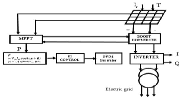
Fig 5: power system and control of the pv connected to the electrical grid (ref. [1]).
