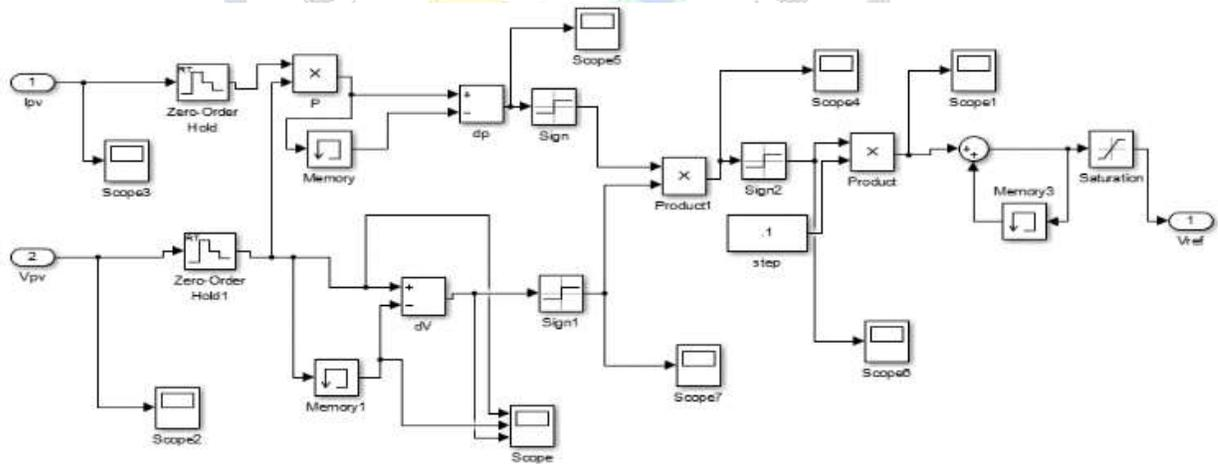
Fig 2: simulation model of perturb & observe mppt technique.
