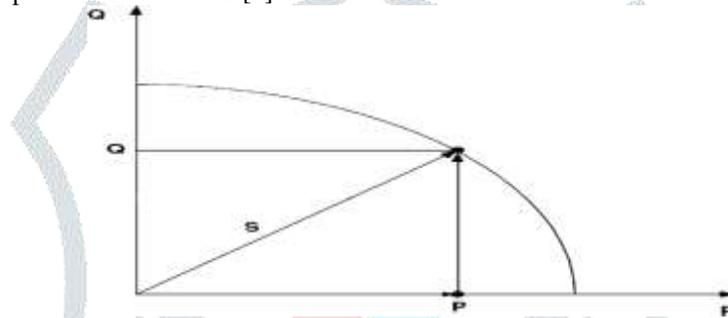
Fig 4: operational modes of inverter.
