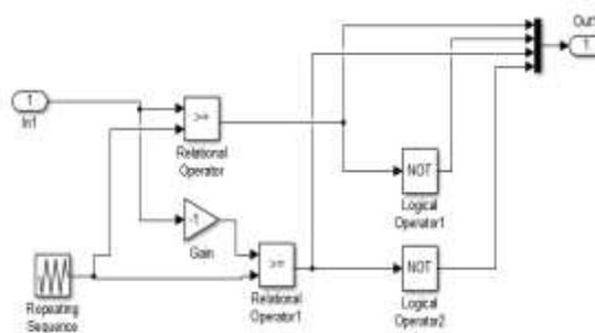
Fig 8: pulse generation block.
