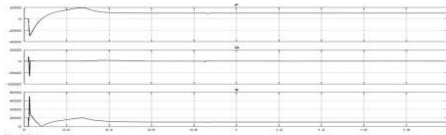
Fig 10: simulation results showing active, reactive and apparent power for 100% insolation.
