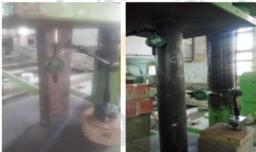
Figure 1 Setup Circular and Square CFST
