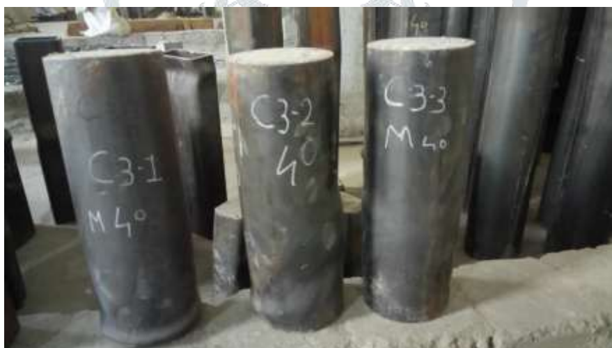
Figure 5 Tested circular CFST
