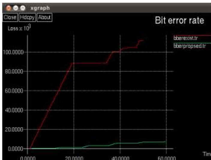
fig 12: bit error rate v/s time
