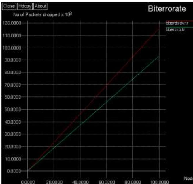
Fig.17 : Bit Error Rate comparison between DSDV and ZRP protocol
