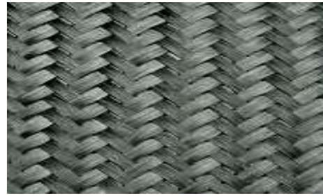
Fig. 8 Carbon Fiber Twill Weave
