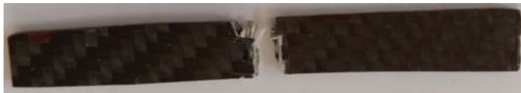
Fig. 15 Specimen after Flexural test.
