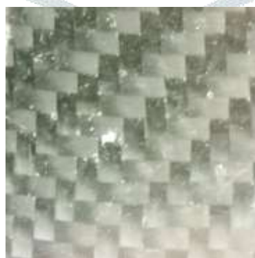
Fig.16 Specimen after Barcol Hardness test(Camera Shot).
