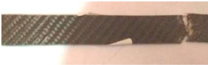
Fig.13 Specimen After tensile testing (Camera Shot).
