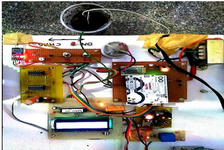
Fig. 10. Testing Soil Moisture, Temperature, Humidity and Illumination System with the Arduino Board
