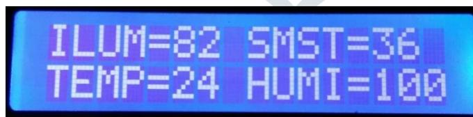
Fig. 11. Results of Soil Moisture, Temperature, Humidity and Illumination on LCD Display
