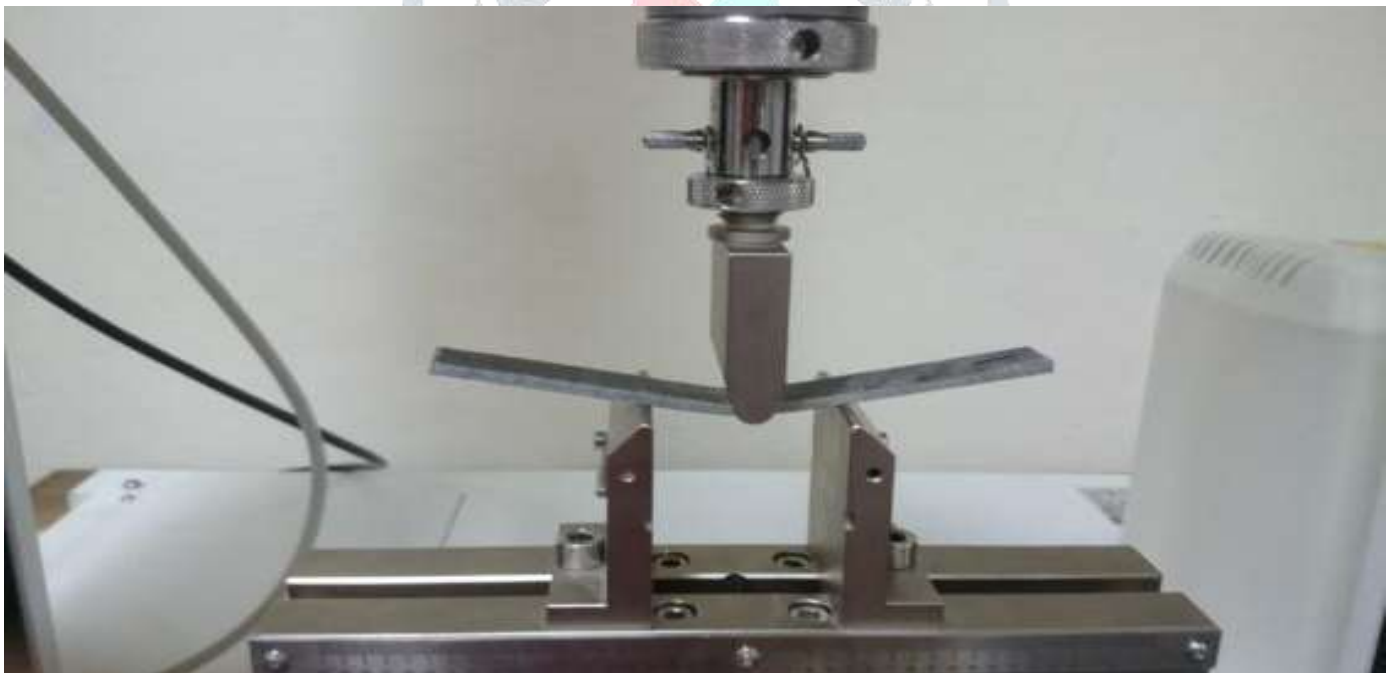
Figure: Experimental setup for flexural testing
