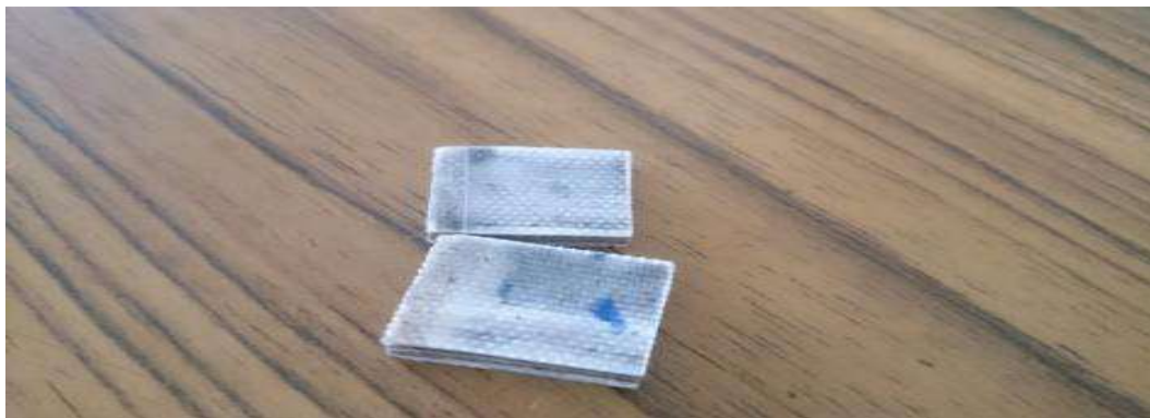
Figure: specimen after compression test.
