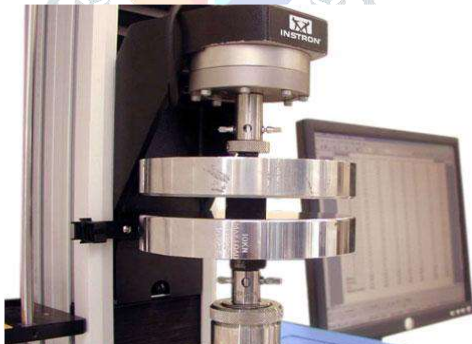
Figure: Experimental setup for compression test
