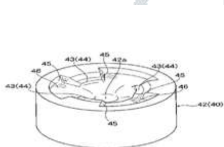
Fig 8: Perspective view of a die unit use in secondary forging step.
