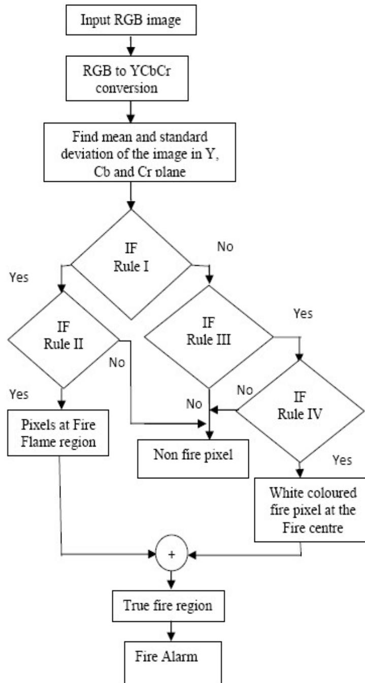
Figure 2. Forest Fire Detection using YCbCr Model
