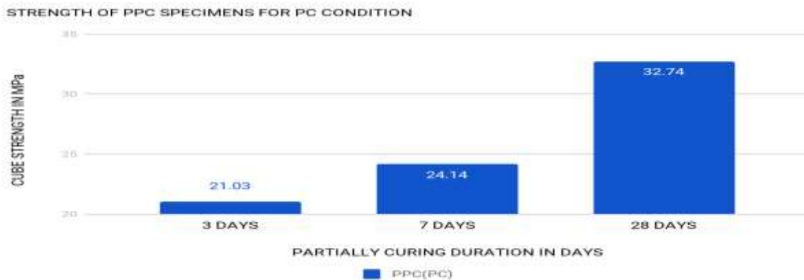
Fig. 11 Cube Compressive Strength of PPC for PC condition
