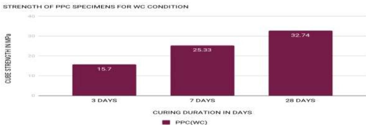
Fig. 8 Cube Compressive Strength of PPC for WC condition.
