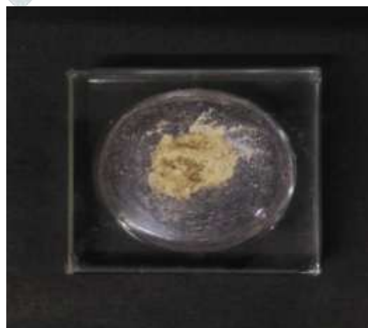
Fig. 3 Photographs showing silk fibroin powder obtained from silk fibroin solutions of (a) Eri and (b) Muga
