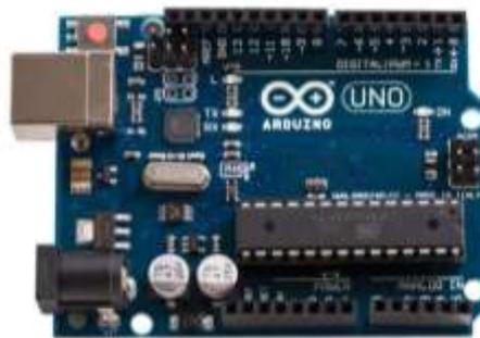
Fig 5: Arduino UNO Board
