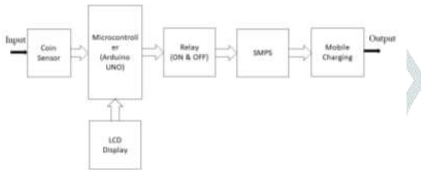
Fig 1: Block Diagram of coin based mobile charging system
