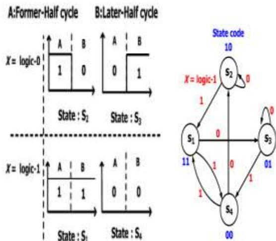
FSM of FM0 suppose the initial state is S1, and its state code is 11 for A and B, respectively.
